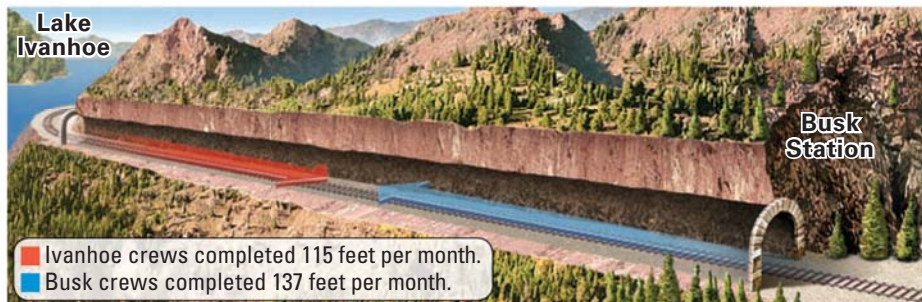
Cutaway of Busk-Ivanhoe Tunnel
