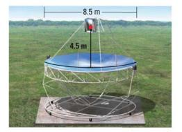
**STEP 1** Write an equation for the cross section. The engine is at the focus, which is |p| = 4.5 meters from the vertex. Because the focus is above the vertex, *p* is positive, so p = 4.5. An equation for the cross section of the EuroDish with its vertex at the origin is as follows:
